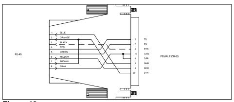
Figure 13: PC, PS/2 Computer/Terminal Adapte
